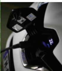
**! LE CÂBLE DOIT ÊTRE COMPLÈTEMENT DÉROULÉ PENDANT LA CHARGE AFIN QU'IL NE SURCHAUFFE PAS.**
